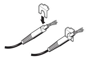
Before inserting the new cable, try out the cable clamp.
