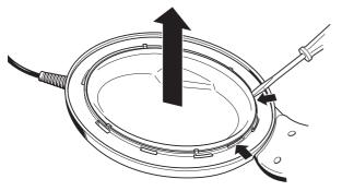
Use a flat screwdriver to carefully lift off the system cover.
