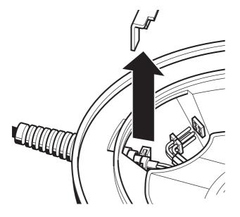
Remove the cable clamp.
