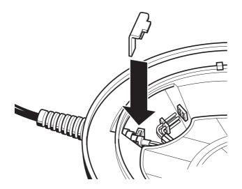
Insert the cable clamp into the notch on the cable.
