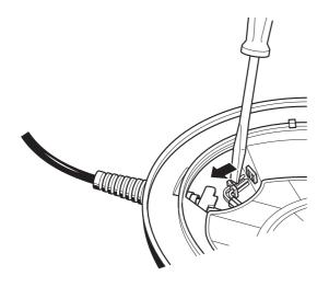
Remove the cable ends from the socket.
