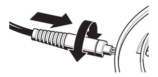
Insert the cable ends into the small hollow space and guide the cable (without the cable clamp) through the opening by turning it to and fro.
