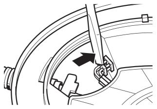
Insert the cable ends into the socket as shown
