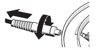
Remove the cable by turning it to and fro.
